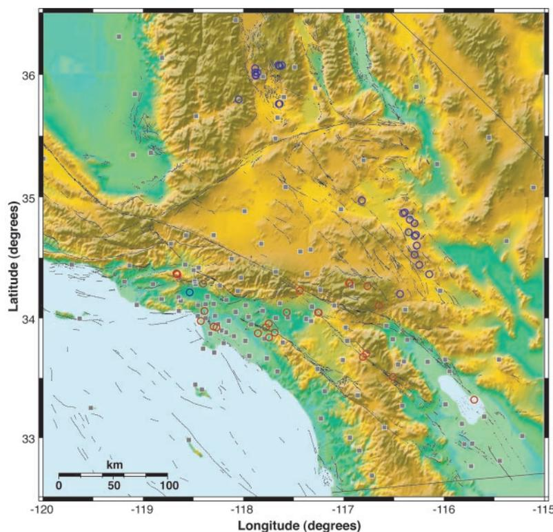
Fig. 2. Tectonic map of southern California showing topography (color scale), mapped fault distribution (thin black lines), locations of the TriNet stations with the necessary real-time capabilities to implement ElarmS (gray squares), and epicenters of the 53 earthquakes used in this study (blue and red circles). The 28 earthquakes used to demonstrate the performance of ElarmS as a function of time are shown in red.
