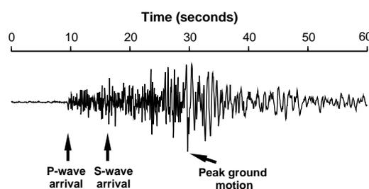
Fig. 1. Typical seismic waveform for a local earthquake. This trace of horizontal ground motion was recorded 50 km from the epicenter of a magnitude 3.9 earthquake in southern California. Indicated are the P-wave and S-wave arrival times and the peak ground motion, which is required to determine local magnitude.
